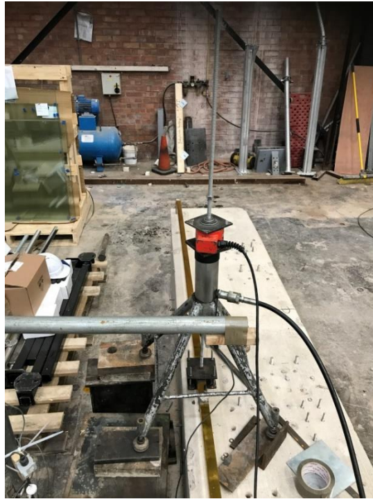
Plate 3 - Top Rail Test Arrangement
