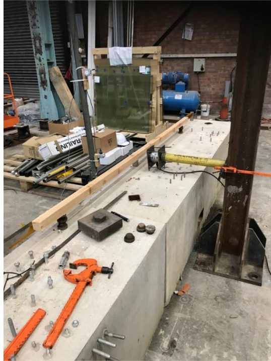
Plate 1 - Bottom Rail under Load
